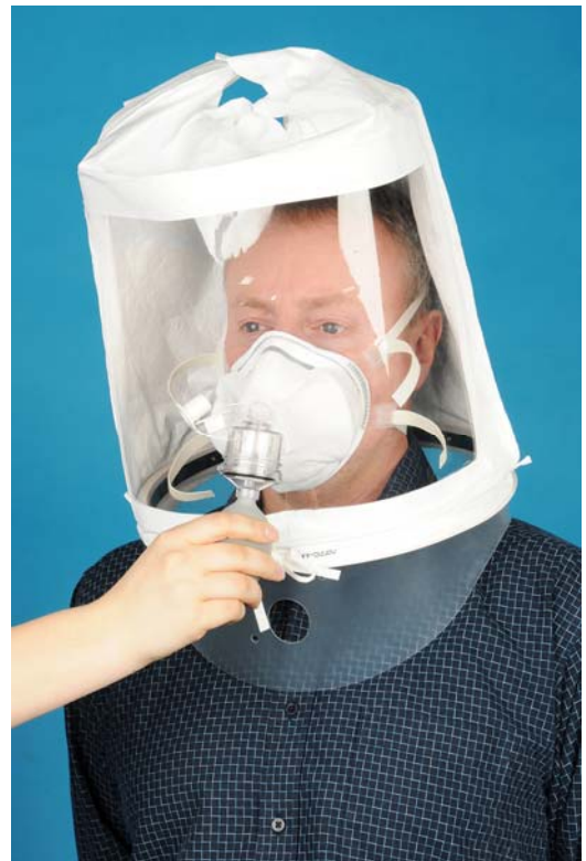
Fig. 7 Example of a qualitative fit test method
