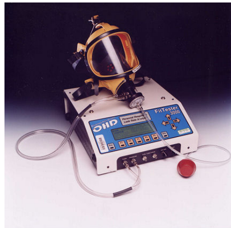
Fig. 10 Controlled negative pressure fit testing device
